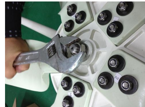
③ Fully tighten the nut to 154N.m
